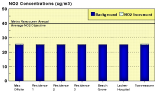
Figure 3 - Predicted Highest Annual Average Total NO x Concentrations at Selected Receptor Locations of Interest
